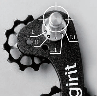
Figure 1 : Grease the mounting pivot.
