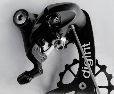
Figure 2 : Mount the tension spring in either the H or L tension setting holes.
