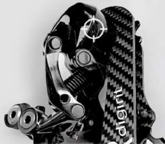
Figure 2 : Mount the tension spring in either the H or L tension setting holes.
